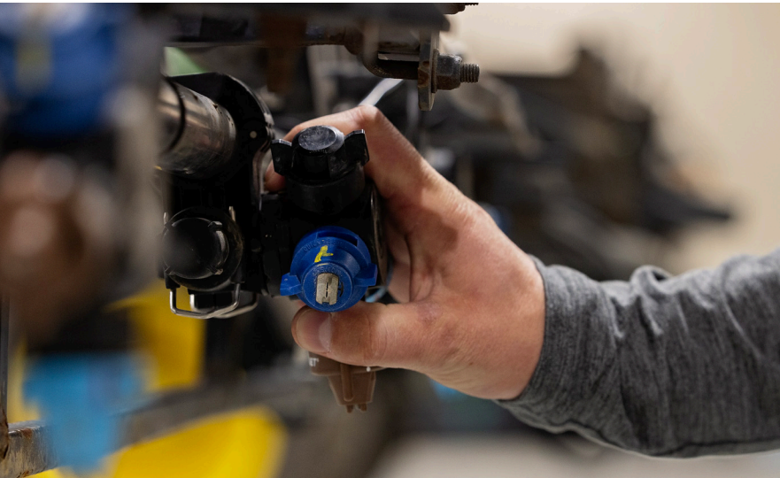
Buildup on spray tips can result in an inconsistent spray pattern.
