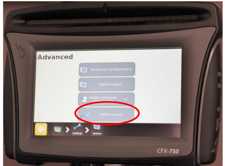
**Step 6:** Now we will tell the Trimble CFX which port to send the NMEA messages through. Available options for external Ports are A & B, select port A.
