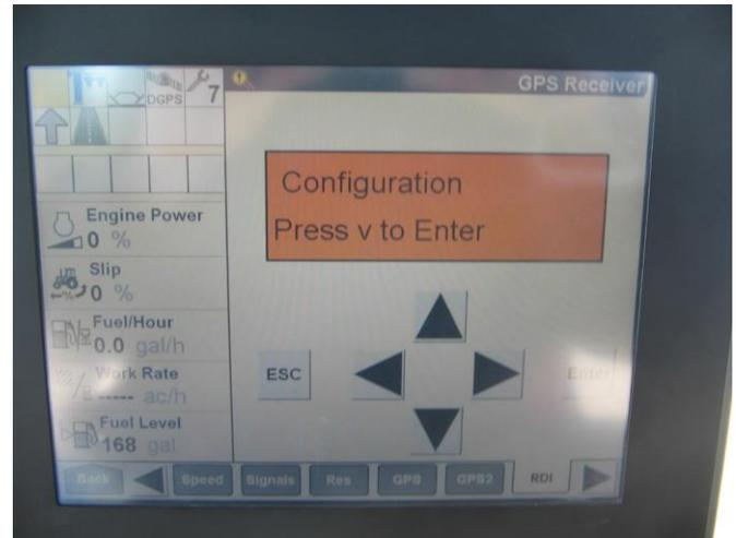
**Step 5:** Push the right arrow until you see the Port A or B or C Config Screen. Then press the down arrow to select which port you have the 727131 harness plugged into. If you have the 727131 plugged into Port B and the harness that was in Port B into the open port on the 727131 use Port C Config.
