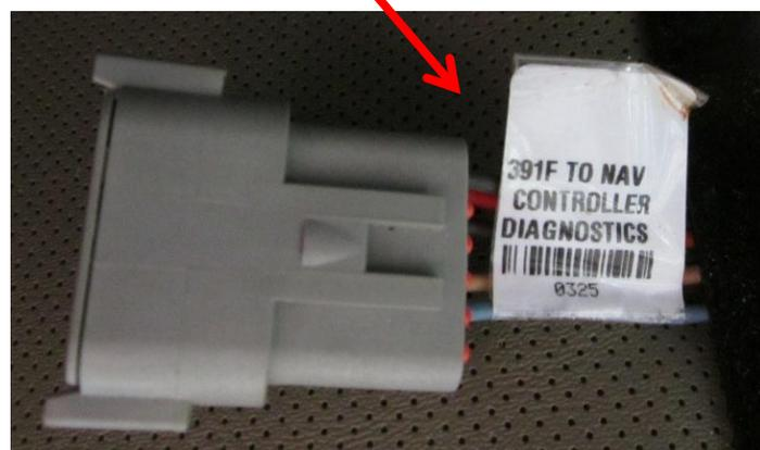
**Step 4:** Connect the 4-pin AMP “GPS Port 1&1 2” to the “GPS” port on the SeedSense tractor harness.
