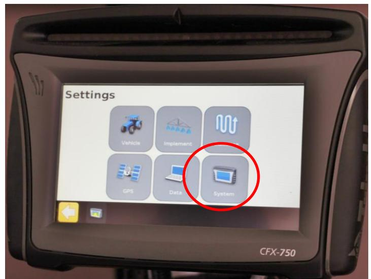
**Step 3:** During this step we will change the user configuration to Advanced. The CFX-750 will not allow the user to output NMEA messages without Advanced User enabled.
