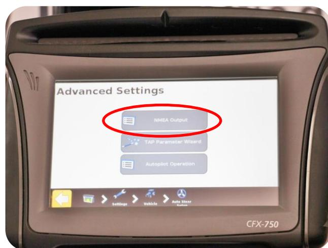
**Step 5:** This screen will set the NMEA Output Parameters. Three critical settings on this screen are needed for GPS to be sent to 20/20.
