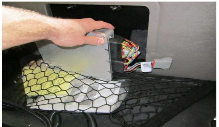
**Step 3:** Connect the 12-pin Deutsch connector on the 727131 Trimble GPS Adapter to the 12-pin Deutsch “Controller Diagnostics”.
