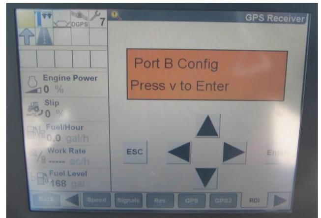
**Step 6:** Click the right arrow to get an active cursor, use right/left arrows to move the cursor to different settings. Move the cursor to the second line next to 8N1 O TSIP and select TSIP. Use the up and down arrows to select NMEA then select baud rate at 38K.4 or 19K.2. Once selected, press the enter button.
