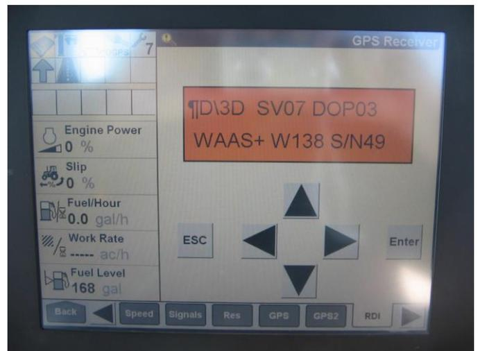
**Step 4:** Press the right arrow until you see the Configuration screen. Then press the down arrow to enter.
