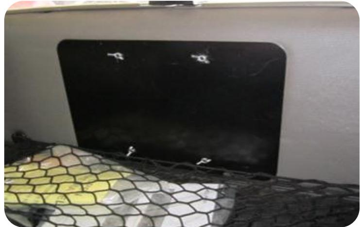
**Step 2:** Slide the NAV II box off of the threaded studs to expose the connectors on its right side. There is a 12-pin Deutsch plug labeled “Controller Diagnostics.”
