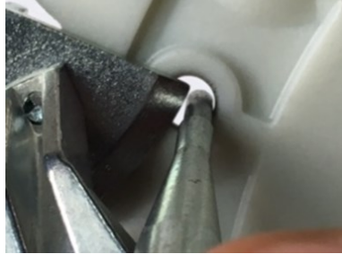
Figure 3a: Lobe clears narrower diameter portion of gauge
